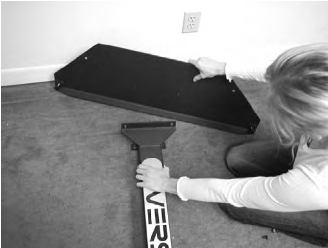
Lay the post on the floor with the large VersaClimber label facing up. Join base plate to post.
